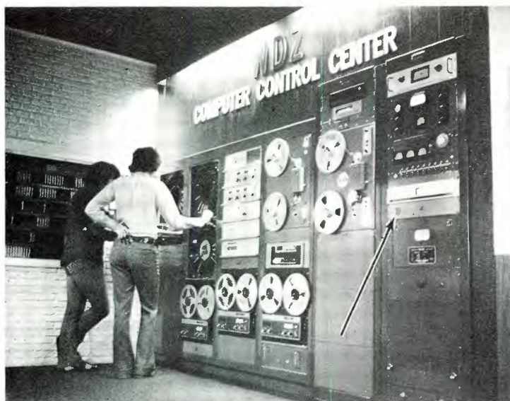
The arrow points to the WDW impatient listener alarm. Such alarms are vital to automated stations.
